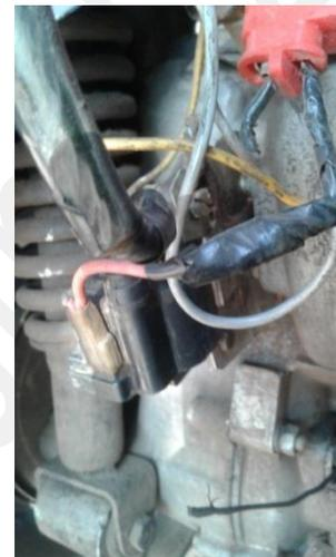
(b) H.T. coil used by a Grasscutter fixed to Two-stroke Scooter Engine
