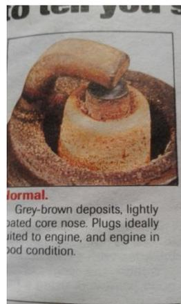
(b) The face of the plug says condition of engine Operation.
