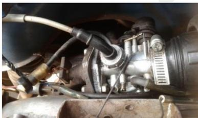
(a) Modified carb fixed to Scooter Engine
